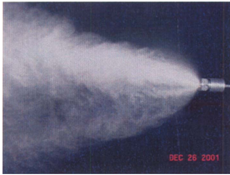
Fig. 8 Distorted spray plume caused by intentional bending of the impaction pin, 138 bar (2000 psi) operating pressure
