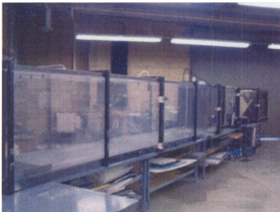
Fig. 2 Experimental wind tunnel, 10.5 m (34.5 ft.) long and capable of velocities up to 25 m/s (4900 ft/min). Used to study droplet kinetics and thermodynamics under conditions similar to gas turbine inlet air ducts.
